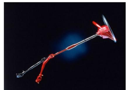
Collapsible steering columns (right) prevent the steering wheel from crashing into the driver. The crumpled zones absorb the force which would otherwise be transferred to the body systems of occupants. With recoiling seat belts and air bags protection (right), the safety cage protects the occupant.
